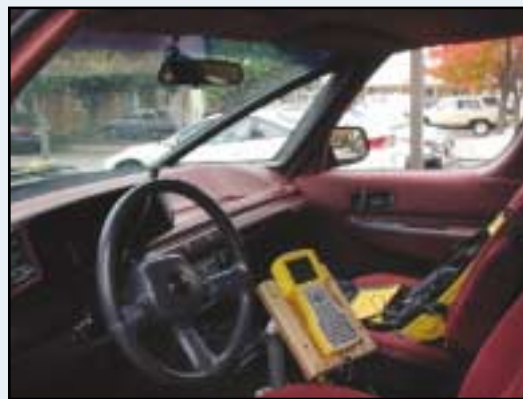
GPS Data Logger equipment used for travel time study
